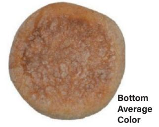
**True color calculations**, on both the top and bottom surface of the product, are measured in various units such as L\*a\*b\*and BCU. The top toast mark may be quantified specifically for size, location, and color, with respect to the whole surface or the central region alone.
