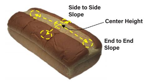
**Profile height calculations** are based on hundreds of individual height values gathered on every product, which leads to a measurement accuracy of  $\pm 0.5$ mm. **Mean Height** is another common measurement applied to bread.
