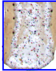
Chipped Corner or Edge (missing perimeter area as compared to a rectangular template)
