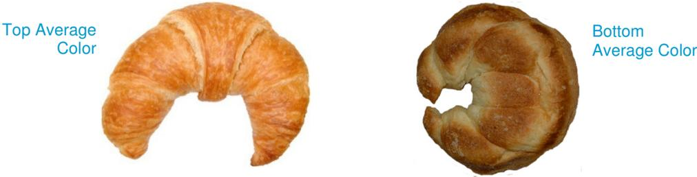
**True color calculations**, on both the top and bottom surface of the product, are measured in various units such as  $L^*a^*b^*$  and BCU.
