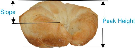
**Profile height calculations** are based on hundreds of individual height values gathered on every product, which leads to a measurement accuracy of  $\pm 0.5\text{mm}$ . **Mean Height** is another common measurement applied to croissants.
