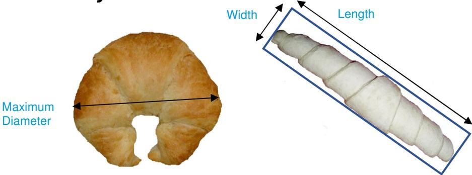
**Two dimensional calculations** are based on an accurately defined perimeter, which is imaged by both overhead cameras. 2-D measurement accuracy is  $\pm 0.5\text{mm}$ . **Mean Diameter**, **Roundness**, **Surface Area**, and **Volume** are other common measurements applied to croissants.
