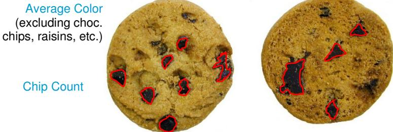
**True color calculations** are measured in various units such as  $L^*a^*b^*$  and BCU, which quantify small variations of bake color.
