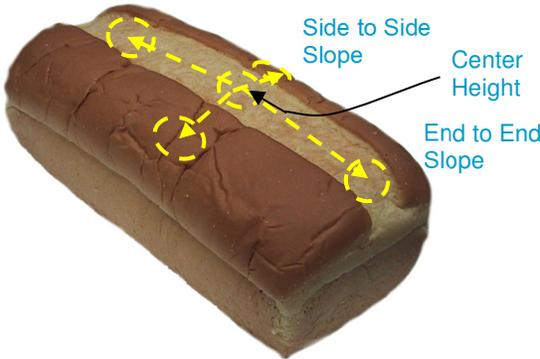
**Profile height calculations** are based on hundreds of individual height values gathered on every product, which leads to a measurement accuracy of  $\pm 0.5\text{mm}$ . **Mean Height** is another common measurement applied to bagels.
