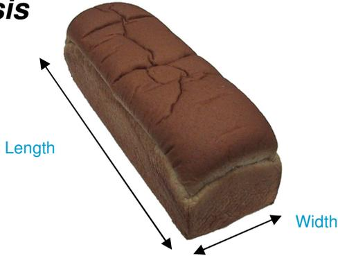
**Two dimensional calculations** are based on an accurately defined perimeter, which is imaged by both overhead cameras. 2-D measurement accuracy is  $\pm 0.5\text{mm}$ . **Surface Area** and **Volume** are other common dimensional measurements applied to bread loaves.
